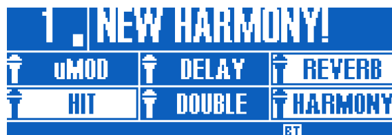
The Home screen with the Backing Track ("BT") indicator
